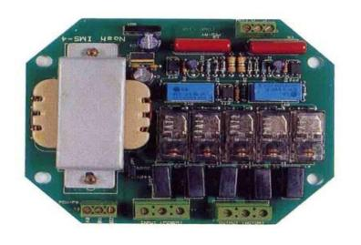
Combined transformer with electric contactor and directly provides various control voltages to the Actuator(24VDC 110VAC/220VAC) from main power (380VAC/440VAC)
