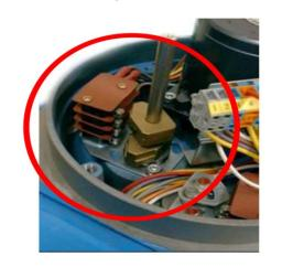
>Providing the dry contact signal to check valve's positions (cam switches structure)
